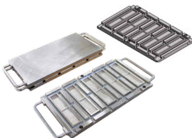
DeMattia flex-fatigue mould (5 cavities)
